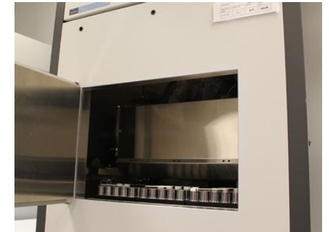
Quantulus Ultra Low Background Liquid Scintillation Counter
