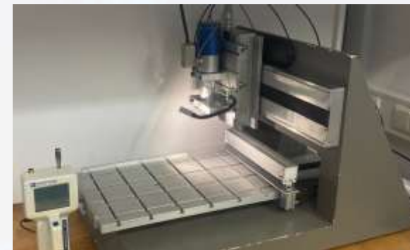
CNC machine placed in laminar flow hood
