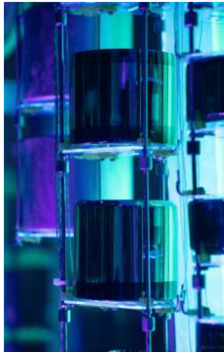
PEN holder plates for enriched Ge detectors
