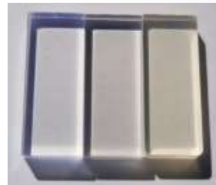
left to right: EJ-200, PEN-C, PEN-G (4 mm thickness)
