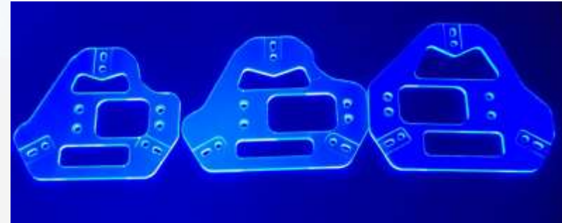
Final components machined for detector holders for LEGEND-200
