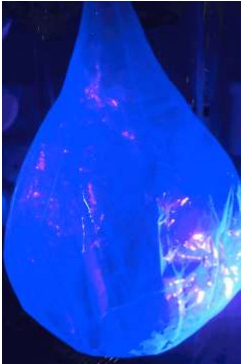
PEN test balloon to hold ^{136}\text{Xe} -loaded liquid scintillator
