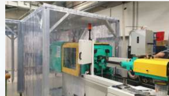
Injection molding machine in cleanroom
