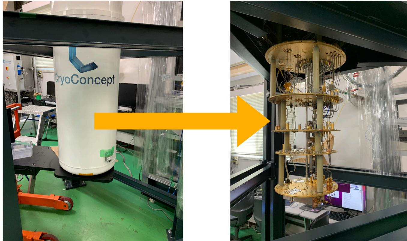
Low-BG cryostat for development of superconducting sensors (KID, TES, etc.) and absorbers for future DM and rare decay search
