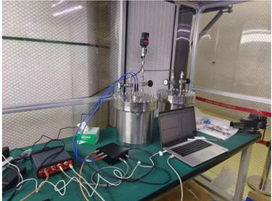
Picture of radon emanation system
