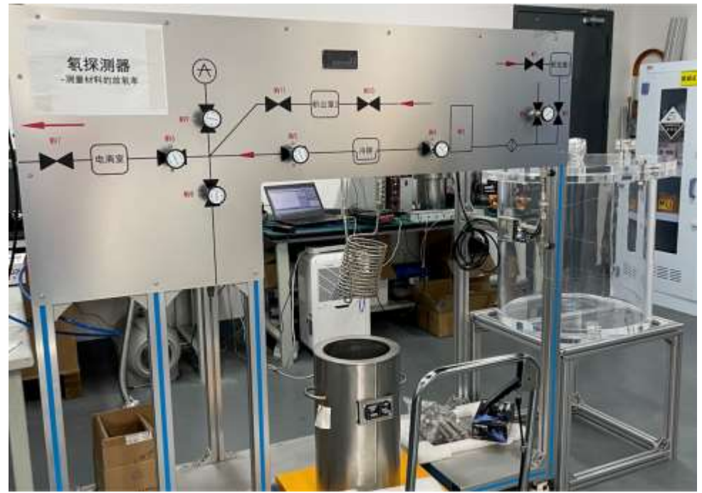
Picture of radon trap system
