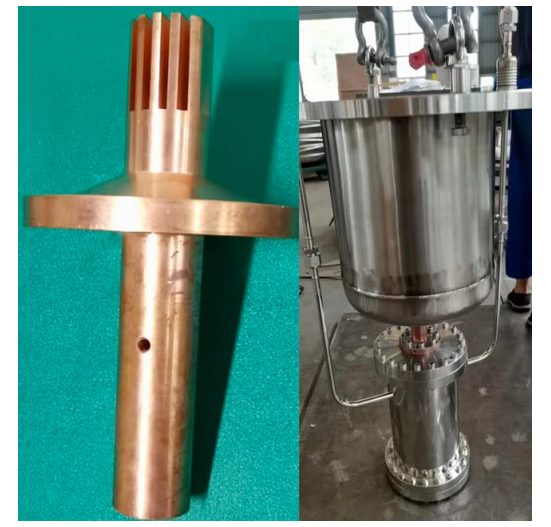
Cold head and the inner structure of enrichment system
