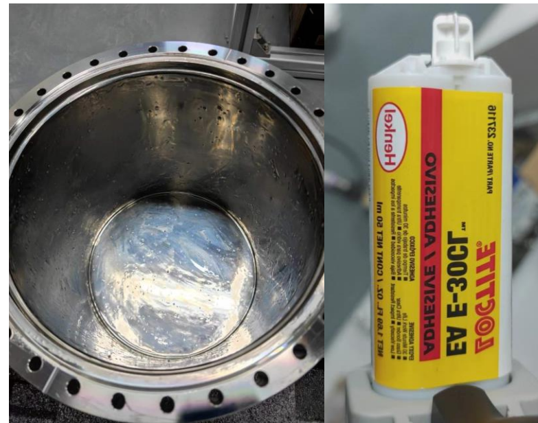
Internal surface after epoxy coating
