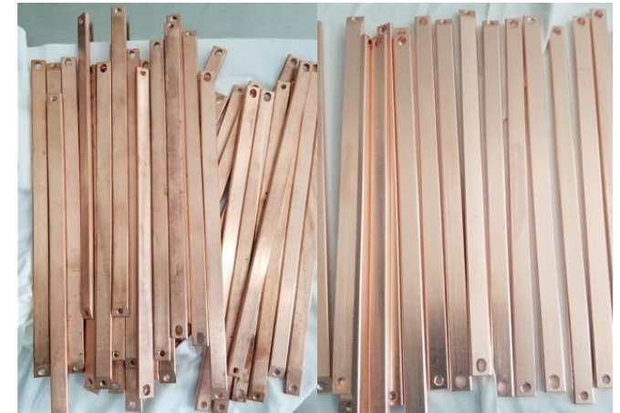
Before(left) and after(right) pickling and passivation copper
